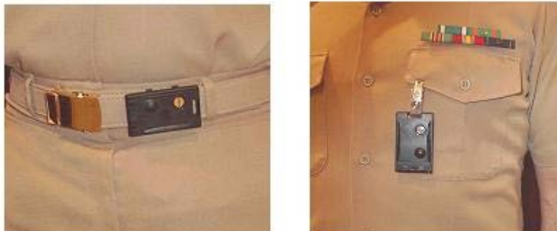
Figure 4. DT-702/PD TLD worn at the waist for neutron exposures and at the chest for non-neutron exposures.
